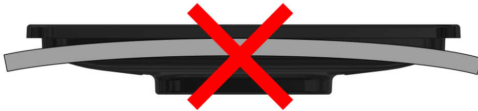
Improper TDU mounting
